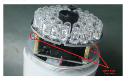
5. Then please close the housing. Please make sure that the rubber ring is straight and not bent or moved. Otherwise, the tightness of the housing can not be guaranteed.
