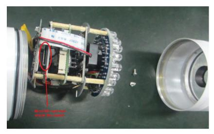
4. Please slide the module back into the housing and secure it with the 2 screws.
